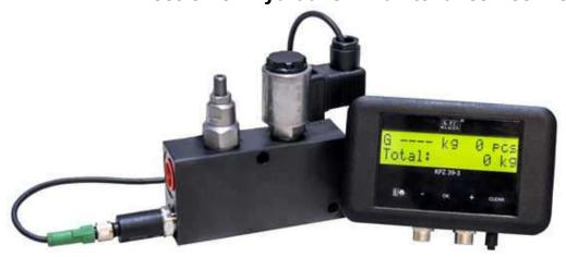
KPZ 39-3 weighing system's operation principle is based on measuring the working machine's hydraulic cylinder pressure. Pressure transmitter reading is automatically scaled to weighing information (kg's or lbs.) and displayed on the operating panel.
