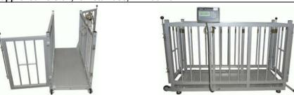
KPZ 2AA, low profile Animal platform scale, dim 560 x 1510 mm, robust and stable, high quality construction of Aluminum with structured plate, Frame height 850mm, with door at the front and back, and wheels for easy transport Load cells: 4 high quality, OIML approved C 3, DMS load cell, IP 67, type KPZ 502E-3. Weighing Indicator: KPZ 52E91, sensible animal Filter. Certification: EU type approved version, for retail use, CE -conform. Capacity: 0 kg, to 300 kg, Division: 100g
