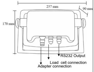
(For IP 67 use only cable diameter from 3 to 5,5mm)
