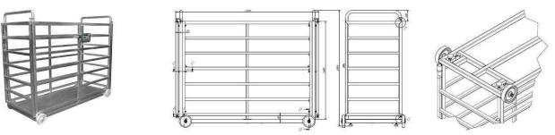
KPZ 2A, low profile Animal platform scale, dim 920 x 2200 mm, robust and stable, high quality steel construction with structured plate, Galvanized version with a galvanized raw framework, Load cells: 4 high quality, OIML approved C 3, DMS load cell, IP 68, type KPZ 502E-3. Weighing Indicator: KPZ 52E91 – sensitive Animal Filter Certification: EU type approved version, for retail use, CE - conform.
