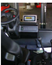
KPZ 39 Hydraulic weighing system
